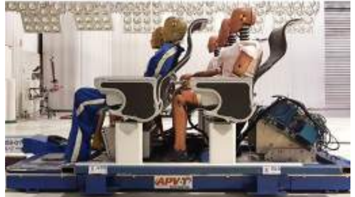
Testing UES Seating products to 6G in Melbourne
